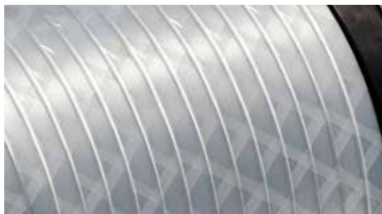
flat enamelled aluminium wire insulated with 2 layers SynTherm® P, in opposite directions, 20 % overlap
