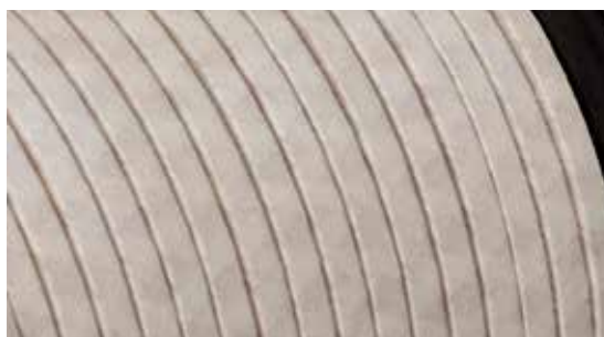
flat copper wire insulated with 2 layers SynTherm® YT510, in opposite directions, 30 % overlap
