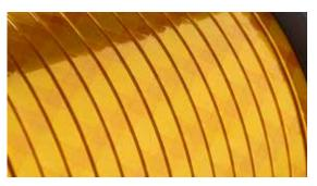
flat aluminium wire insulated with 2 layers SynTherm® H, in opposite directions, 25 % overlap
