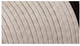
flat copper wire insulated with 2 layers SynTherm® YT510, in opposite directions, 30 % overlap
