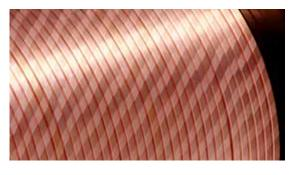
flat copper wire insulated with 1 layer SynTherm® P, 30 % overlap
